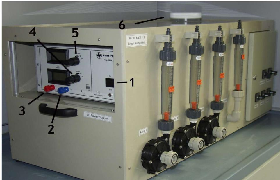
Fig. 4: The power supply and position of electrolyte container in PCCell B-ED 1.
