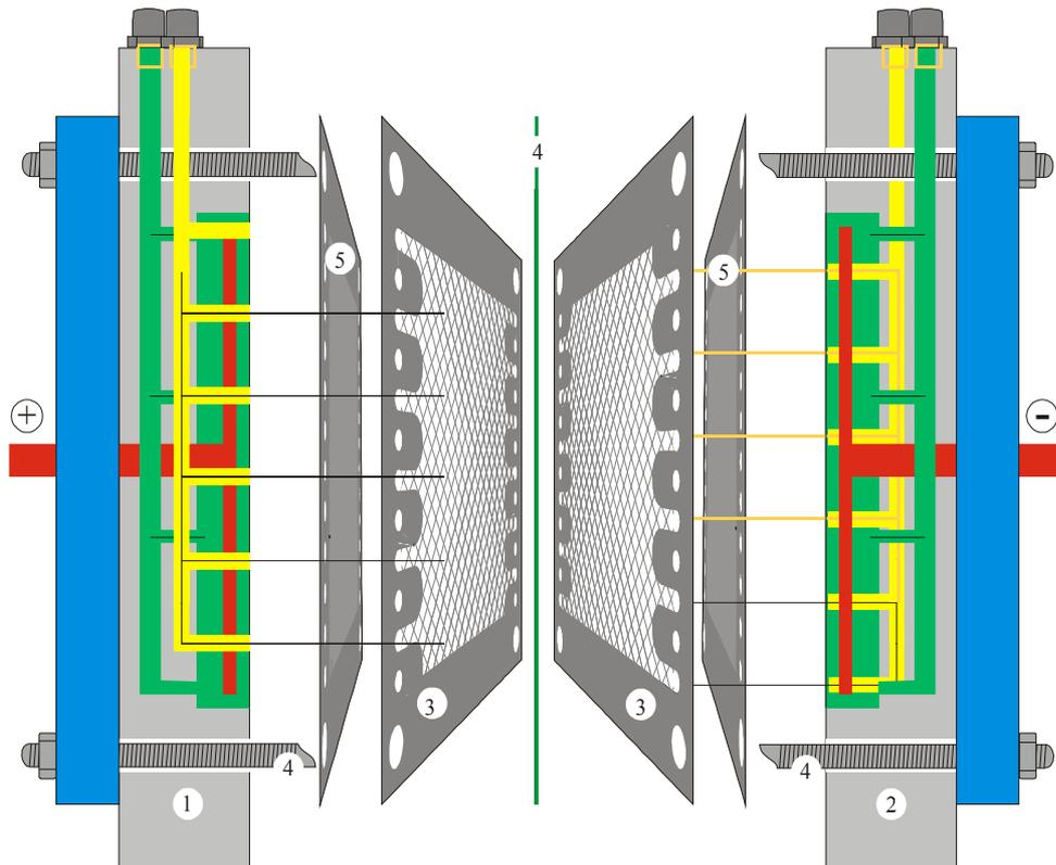
Fig. 3: PCCell ED 64 setup and functional parts
