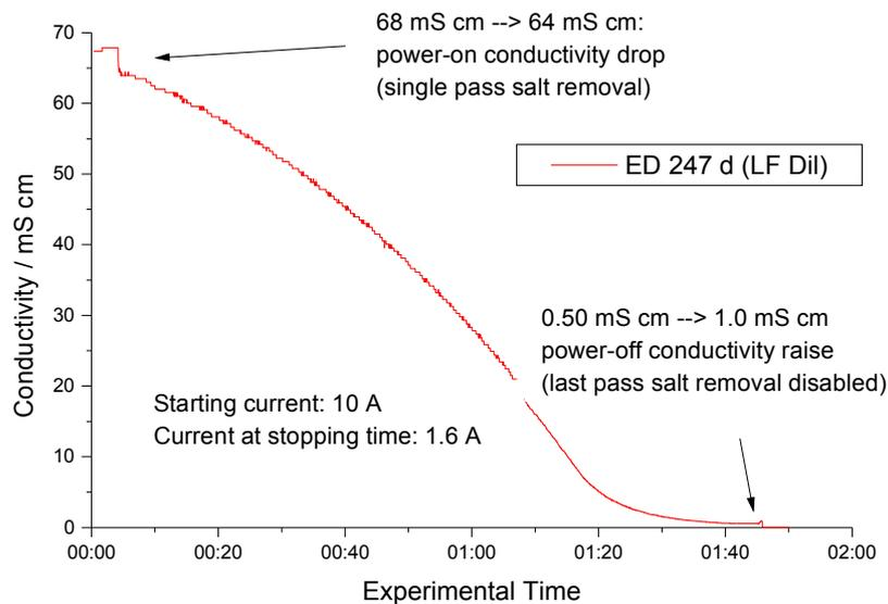
Fig. 6: A batch desalination of aqueous NaCl, about 14 l / m<sup>2</sup>.
