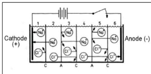
Figure 2. Electrodeionization Stack
